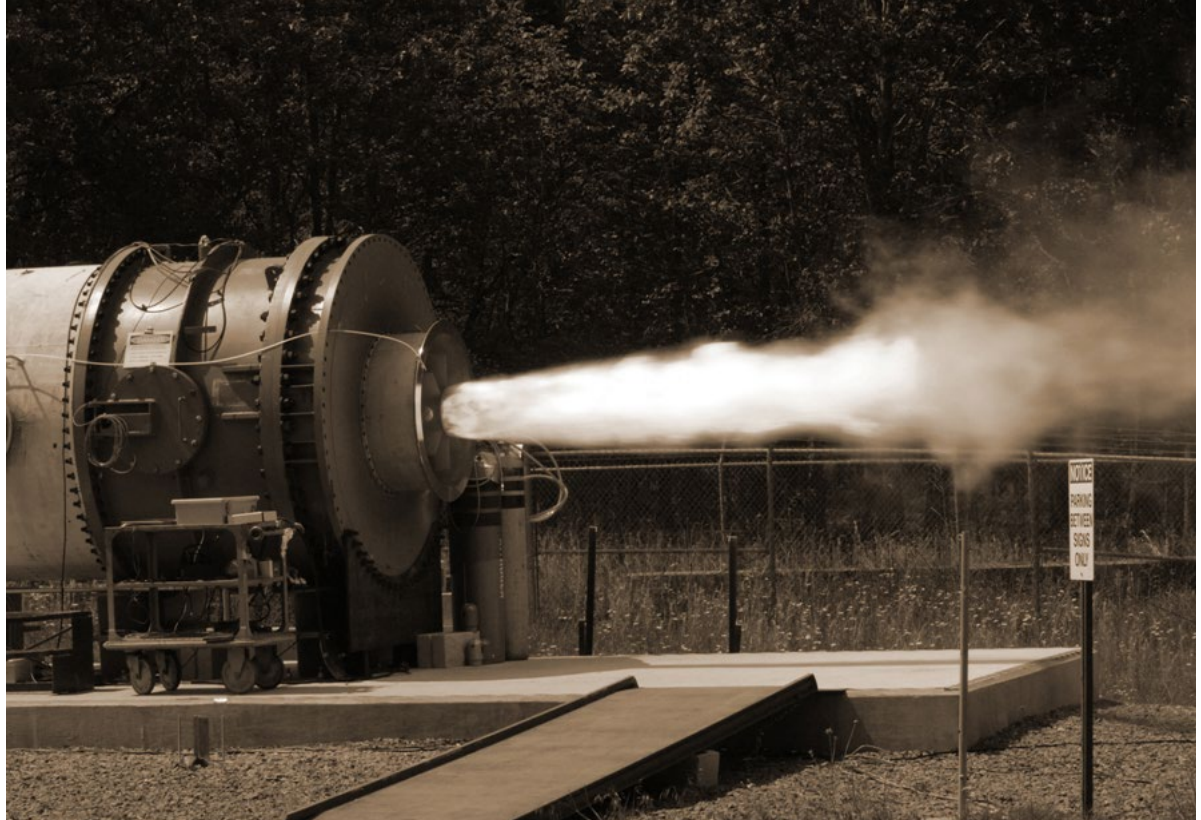
Towed Airborne Plume Simulator being tested at AEDC. (Photo by David Housch)
