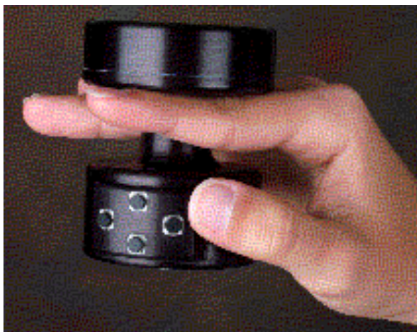
Figure 2. Dual-mode stethoscope used in experiments.
